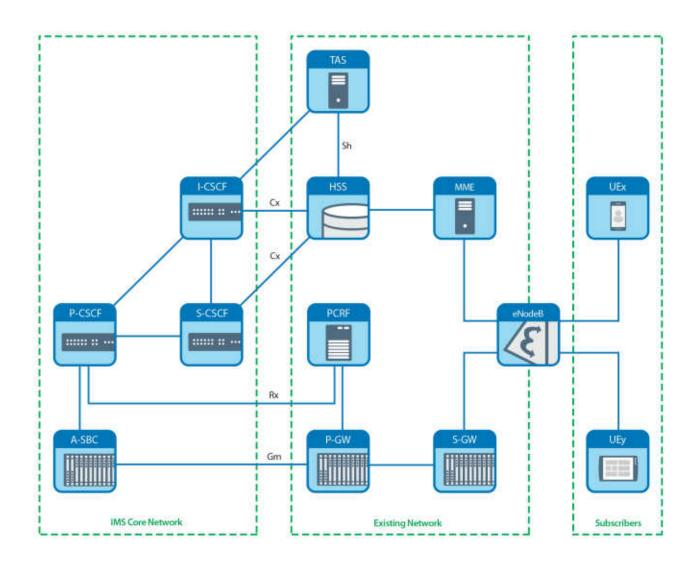
**IMS CSCF (Call Session Control Function)** is intended to provide the registration procedures of terminal equipment and SIP routing.
